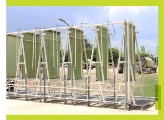
At the Cartagena Plant, we began the process to capture CO<sub>2</sub> with microalgae and its subsequent transformation into biocrude to produce a renewable diesel
